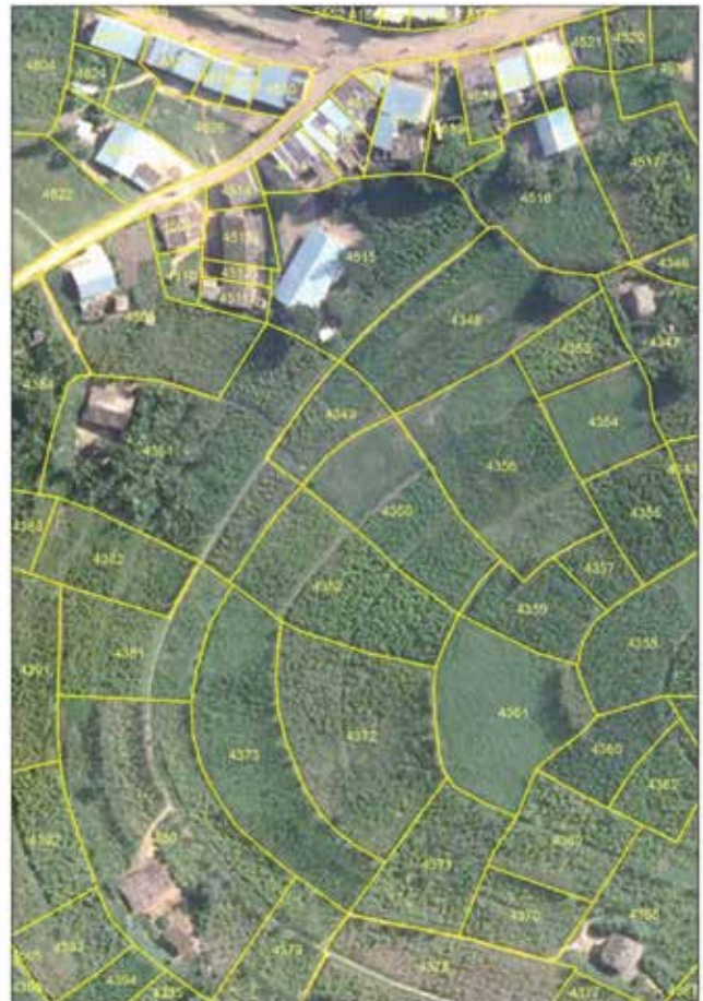
Map 4.1: Example from Rwanda showing aerial imagery (left) from which the parcel boundaries are easily identified (right). Source: Didier Sagashya, Rwanda.
